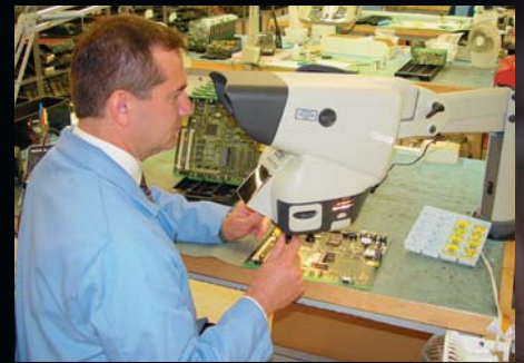
Microscopic review assures consistent SMT and thru-hole assembly
