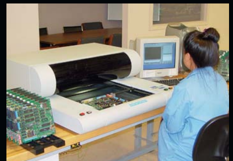
Precise optical inspection verifies components and orientation
