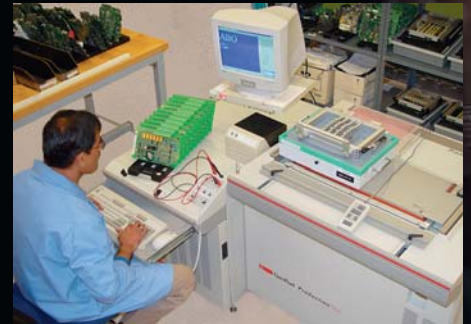
Youngtron's GenRad testing system confirms circuit integrity
